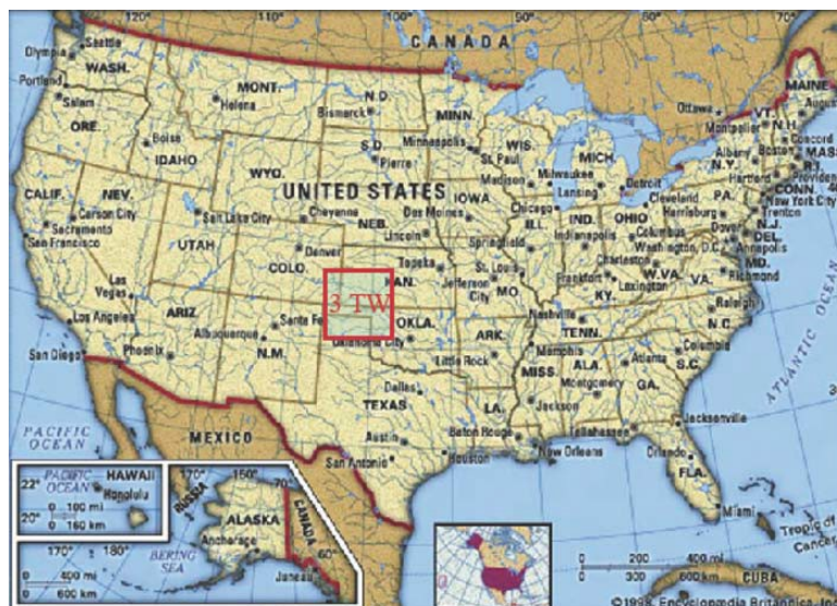
Figure 1.6 –Map of the U.S. (right) with the red square showing the amount of land needed for a solar energy farm operating at 10% efficiency to produce 3 TW of power
