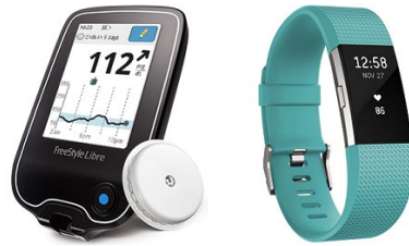
Figure 3.1: On the left the Abbott FreeStyle Libre intermittently scanned Continuous Glucose Monitoring (isCGM) system, while on the right the Fitbit Charge 2 personal fitness tracker (PFT).
