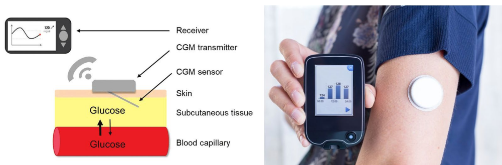
Figure 2.4: On the left a schema of continuous glucose monitoring (CGM) system [33], which measure glycemia in interstitial fluid, and on the right a CGM device in use.
