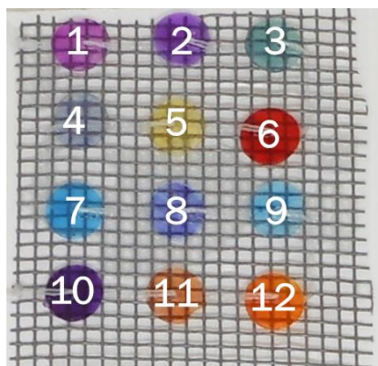
Figure 4.4: Example of 3x4 sensing array used as chemometrics-assisted litmus test. Dye-EVOH@ sensors are numbered from 1 to 12, according to the numbering in Table 4.2
