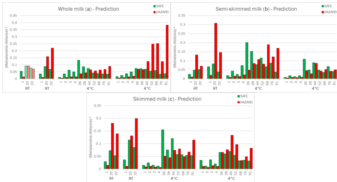
Figure 3.17: Results of prediction of test samples for whole (a), semi-skimmed (b) and skimmed (c) milk, stored at different temperatures, reporting storage time and temperature on the x-axis and the inverse of Mahalanobis distance from each of the two classes on the y axis.
