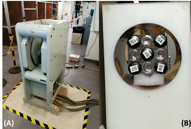
Figure 59: (A) The resistive biplanar 0.1 T MRI system (Bouhnik S.A.S., France). (B) Disposition of the vials inside the bore of the transmitter/receiver coil.
