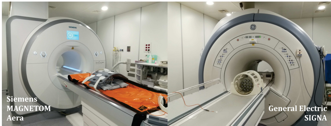
Figure 31: The 1.5 T MRI scanners used in this study: a Siemens Magnetom Aera (left) and a GE Signa (right).
