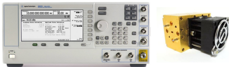
Figure A.6: Automatic external signal generator with high output power produced by Agilent (left) and integrated amplifier/multiplier chain produced by Virginia Diodes (right).
