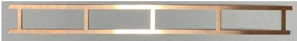
Figure 3.12: Copper compensating structure made through punching technique for IDEM1. The same strip can compensate vertical and horizontal polarizations.
