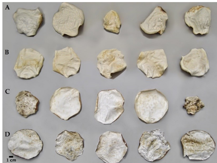
Figure 2. Dry mycelial mats obtained by Mogu's patented method after 3 weeks of growth in Petri plates; five repetitions were conducted per strain: (A) Fomitopsis iberica (10), (B) Daedaleopsis confragosa (6), (C) Corioloopsis gallica (3), and (D) Terana caerulea (19).
