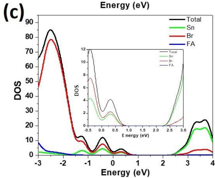
**Figure 3.** Density of states (DOS) of cubic (a)  $\text{FAPbBr}_3$ , (b)  $\text{FAPb}_{0.50}\text{Sn}_{0.50}\text{Br}_3$  (d) and (c)  $\text{FASnBr}_3$  as calculated by HSE06-SOC. Valence band maxima has been set to zero in (a) and (b) and (c) have been aligned to the lowest carbon DOS peak.
