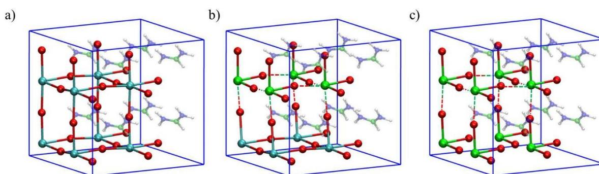
**Figure 4.** Optimized structures of cubic (a)  $\text{FAPbBr}_3$ , (b)  $\text{FAPb}_{0.50}\text{Sn}_{0.50}\text{Br}_3$  (d) and (c)  $\text{FASnBr}_3$ . The dashed lines indicate long Sn-Br distances. Pb=light blue; I=red, Sn=green. FA molecules are shaded in the background for clarity.
