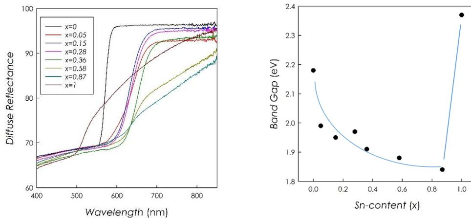
**Figure 2.** a) Diffuse reflectance spectra for the  $\text{FAPb}_{1-x}\text{Sn}_x\text{Br}_3$  system. b) Band-gap trend as a function of Sn content ( $x$ ).
