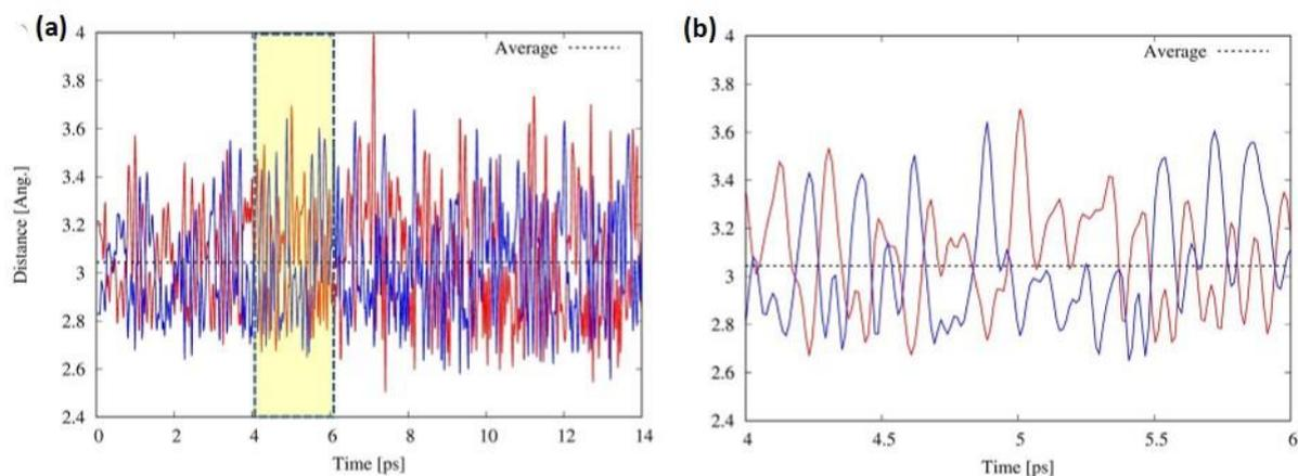
**Figure 5.** Time evolution of Sn-Br bond distances for a selected Sn center along the [001] direction. The right panel shows a detail of the time from 4 to 6 ps highlighted by the yellow rectangle on the left panel.
