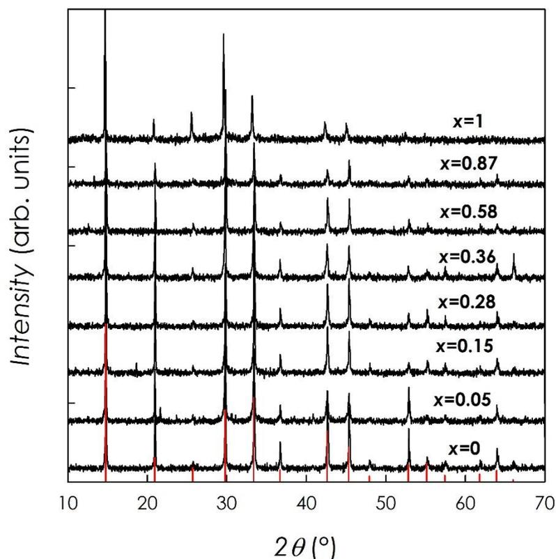
**Figure 1.** XRD patterns for the samples of the  $\text{FAPb}_{1-x}\text{Sn}_x\text{PbBr}_3$  system. Patterns are vertically shifted to clarify viewing. Red vertical bars refer to the reflection positions for cubic structure ( $Pm-3m$ ).
