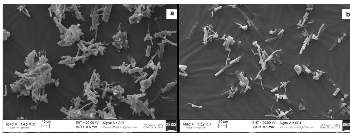
Figure 3. SEM micrographs of the P:PVPel (a), and P:SOLEl (b) samples after milling.
