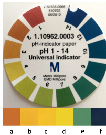
Figure 13. pH color chart of the commercial Litmus paper and color of the Litmus paper after contact with the real samples: a) Schweppes, b) sprite, c) White wine vinegar, d) Tropical aloe vera, e) Tap water, f) ammonia cleaner.
