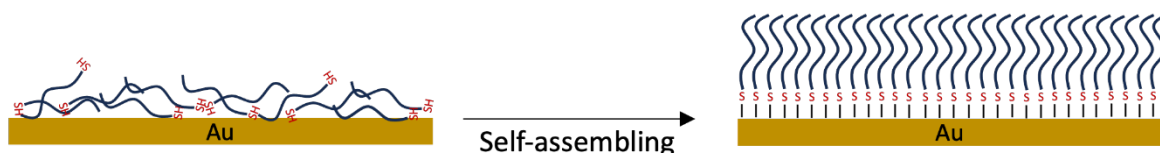
Figure 30. Schematic representation of a self-assembly of thiol molecules on a gold substrate.
