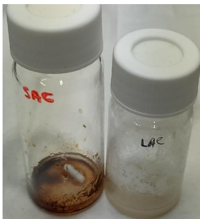
Figure 1: Transesterification of saccharose (sac) and lactose (lac) with vinyl palmitate (VP) using lactic acid as catalyst at 120 °C
