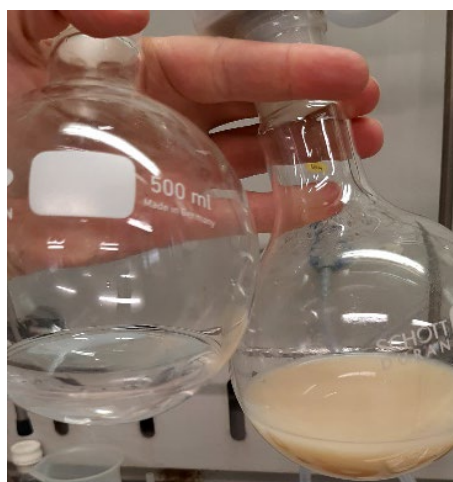
Figure 3: Synthesis of GPI by the mono-enzymatic hydrolysis of ENSL catalyzed by PLA1 in fully aqueous medium. Reaction mixture before (right) and after (left) filtration on the Celite pad
