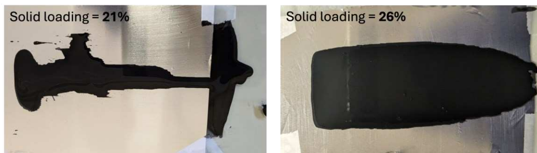
Figure 3. Experimental photos collected after casting anodic slurry with a 90:5:5 (HC:binder:carbon) composition, prepared with different solid loadings, on the Al current collector
