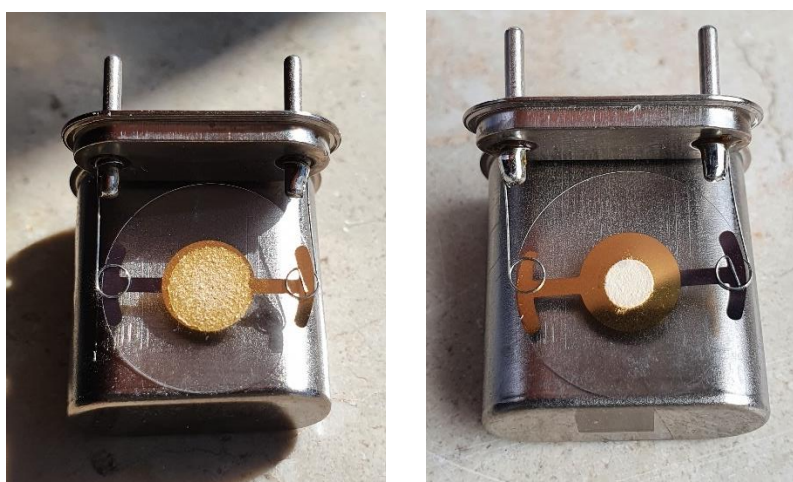
Figure 81 Silica gel powder functionalized gold electrodes QCMs, on the left full electrode functionalization (1 mg deposited), on the right partial functionalization of the electrode (0.3 mg deposited).
