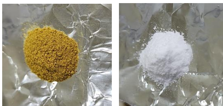
Figure 71 7 nm doped Silica gel powder before (left) and after the removal process with nitric acid (right).
