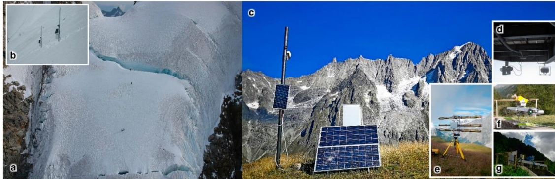
Figure 2. (a) Alpine guides install reflective prisms onto the Whymper Serac on 5 March 2020. (b) GNSS equipped with datalogger, solar panels, and batteries [46]. Reflective prisms were placed on the metallic bars that supported the GNSS for comparison. (c) TLC station that monitors the Montitaz Lobe, with the Planpincieux and Grandes Jorasses glaciers visible in the background. (d) TLC station that monitors the Whymper Serac from Pointe Helbronner. (e–g) the RAR GPRI and the GBSARs IBIS-L and FastGB SAR, respectively.
