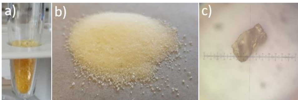
Figure 42. Images of the Bulk-MIP-DVB-DBDS a) after polymerization in the oven; b) ground; c) ground powder by an optical microscope with 10x magnification.
