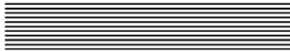
Figure 80. The layout of the printed silver nanoparticles lines (the length ( L ) is 5cm, the spacing ( S ) is 500 \mu m and the width ( W ) is 300 \mu m).
