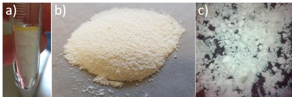
Figure 44. Images of the Porous-MIP-DVB-DBDS1 a) after polymerization in the oven; b) ground; c) ground powder by an optical microscope at 10x magnification.
