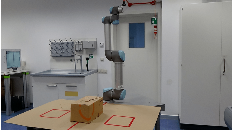
Figure 12.1: The experimental setup used in the case study, made of UR5 manipulator and obstacles
