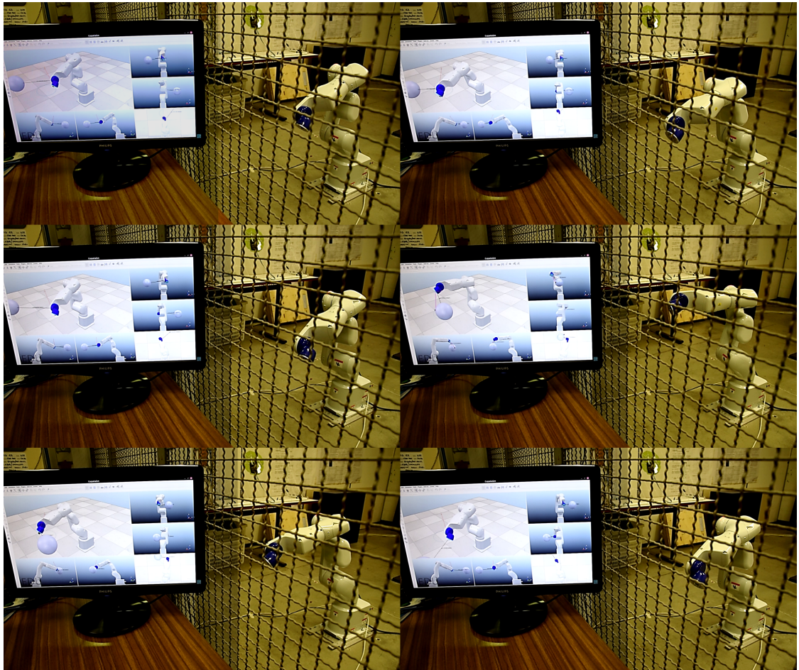
Figure 13.10: Some frames of the experiment described. On the monitor on the left, the virtual robot controlled by the algorithm in Chapter 11 is performing the task, while the real robot mimics it.
